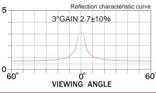
Reflection characteristic image of a wide gradation type (HDR scre
